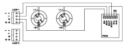
Complete loop wiring. Installation of sensor bases at this time is acceptable. If using a high voltage testing device to verify ground isolation, do not expose devices or modules to the high voltage. Verify wiring per the following:
